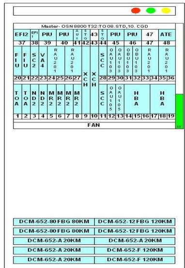
FIGURE 2 – Duplication of essential parts in the network elements
