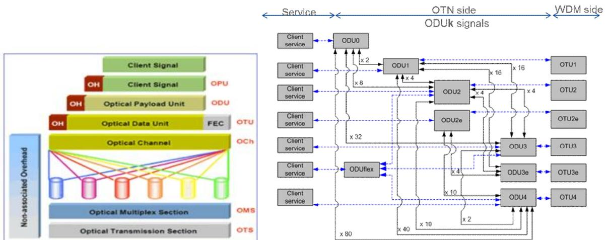
FIGURE 5 – Multiplexing structure and terminology of OTN frame
